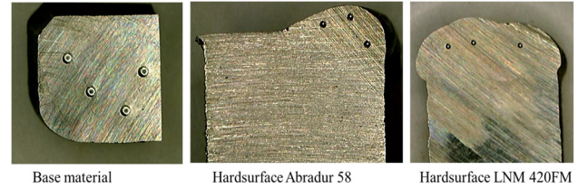
Fig. 6 Measuring hardness of base material and hardsurfaces Source: [1].
