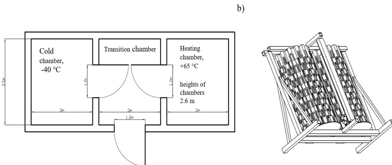
Fig. 2. Bench scheme: a) climatic chamber, b) a set of simulation tanks
