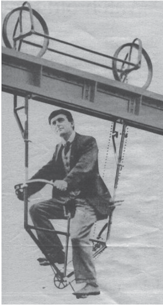
Fig. 2. Suspended monorail bike [4]
