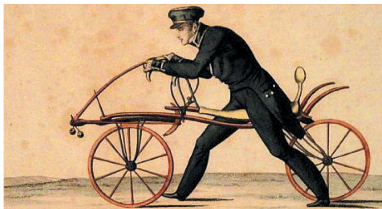
Fig. 1. “Draisine”, Karl Drais' balance bike [3]
