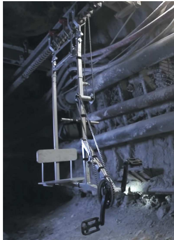
Fig. 17. New miner’s bike prototype in an underground working
