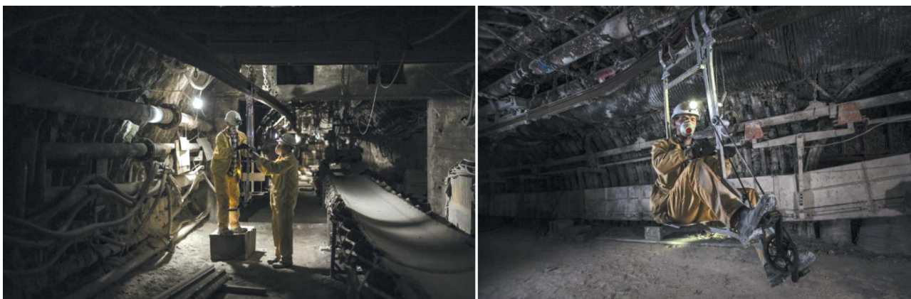
Fig. 18. Underground tests of a new miner's bike
