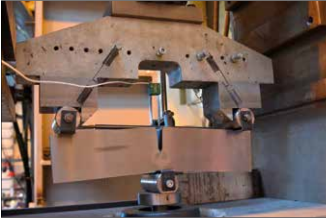
Fig. 9. W100 Specimen during laboratory testing—breaking phase
