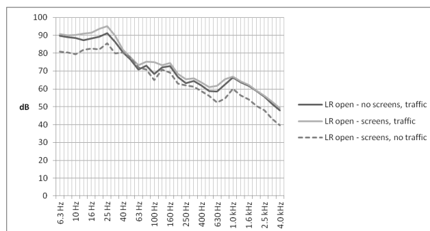
Fig. 3. Background levels in the car cabin for LR open in three measurement variants
