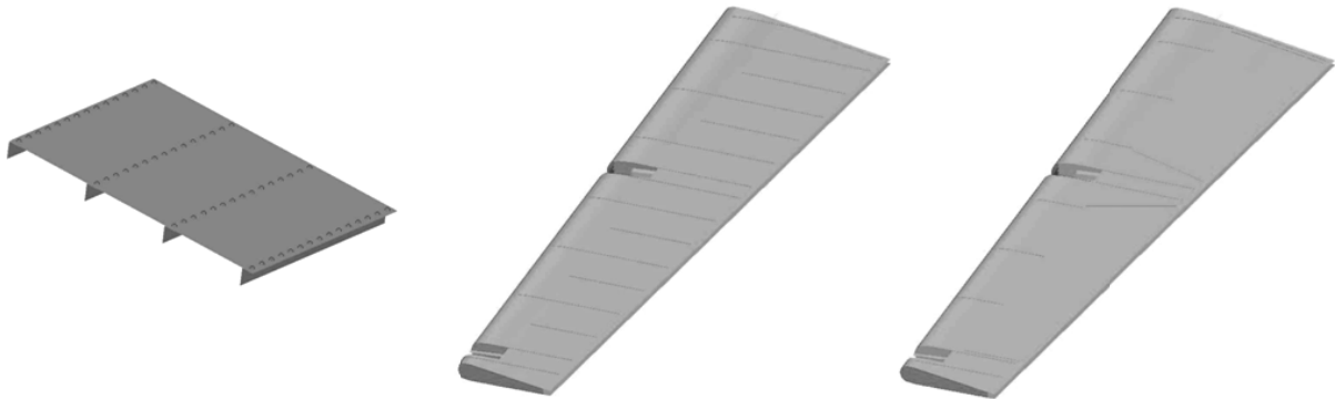
Fig. 3. Model views: the empenage sample (left) and elevator of the classical design (middle) and the honeycomb core design (right). The lines of division into elements are removed
