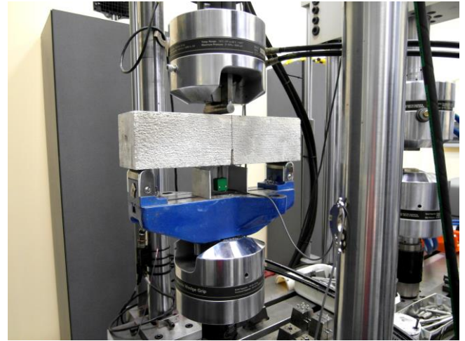
Fig. 2. Notched beam specimen during testing.
