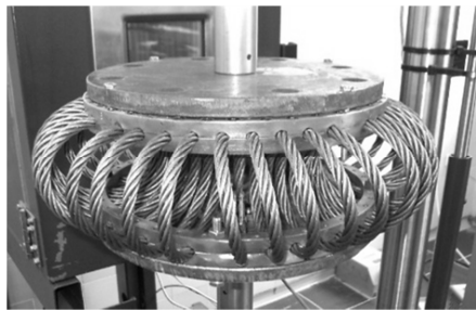
Fig. 6. Ring wire rope absorber
