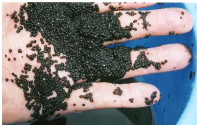
Fig. 1. Anaerobic activated sludge in the form of pellets [3] Rys. 1. Beztlenowy osad czynny w formie granul [3]
