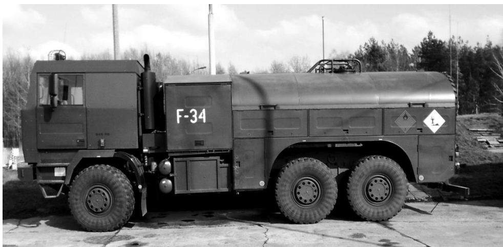
Fig. 6 Tanker distributor with a capacity of 10,300 l (CD-10) for the transport and distribution of aviation fuel on the JELCZ 662 chassis operated by the Armed Forces
