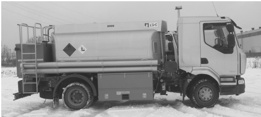
Fig. 3. Tanker distributor with a capacity of 8.900 l (CD-9) for the transport and distribution of aviation fuel on a RENAULT 4x2 chassis operated by the Police
