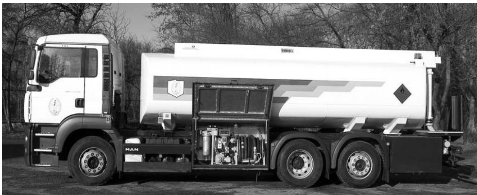
Fig. 2. An 18,000-litre transport tanker (CT-18) with the possibility of distributing aviation fuel to aircraft on a 6x2 MAN chassis operated by the Border Guard
