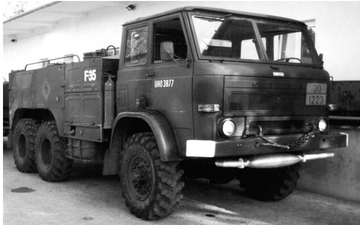
Fig. 5 Tanker distributor with a capacity of 4,500 l (CD-5) for the transportation and distribution of aviation fuel on the STAR 266 chassis, operated by the Armed Forces
