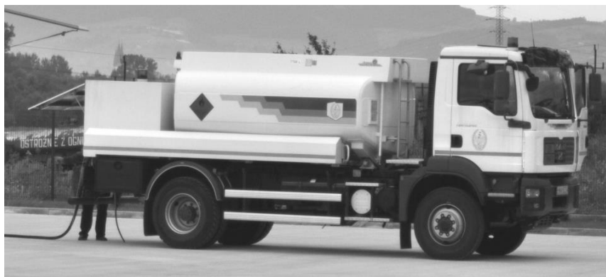
Fig. 1. Tanker distributor equipped with a MAN 4x4 chassis, with a capacity of 7,500 l (CSDL-7) for the transport and distribution of aviation fuel, operated by the Border Guard
