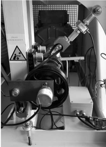
Fig. 1. Research stand for measuring friction in a belt transmission
