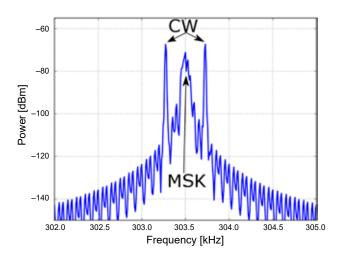
Figure 1. Power spectrum of the radio beacon's R-Mode signal
