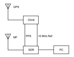
Figure 2. Block diagram of the SDR based R-Mode receiver
