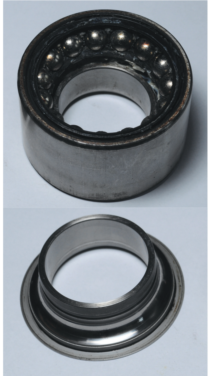
Fig. 3. Bearing VKBA 6831 with inside track
