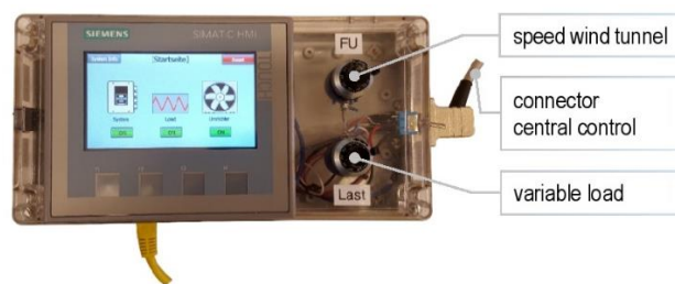
Fig. 6. Remote control of wind tunnel and central control unit
