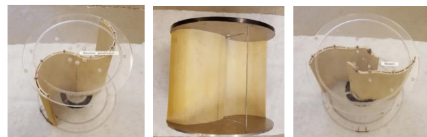
Fig. 3. Vertical rotors: Standard-Savonius rotor (left), J-blade rotor (middle) and Benesh-V Rotor (right)
