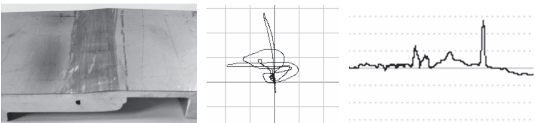
Figure 10. Arc welded specimen with a rough surface and welded plates displacement (a) and EC signals created by subsurface lack of fusion ( b_l = 3 mm) and noise in the impedance complex plane (b) and in time base mode (c).
