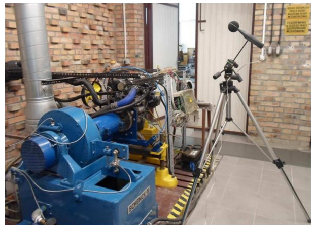
Fig. 1. Test rig for acoustic measurements.
