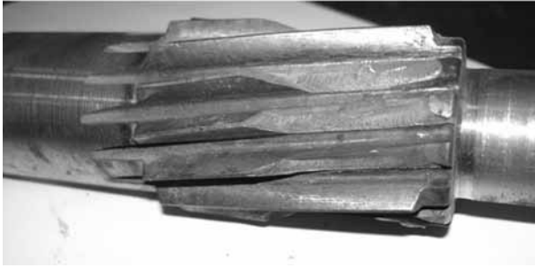
Fig. 1. View of the gear with broken teeth after exploitation in a coal mine
