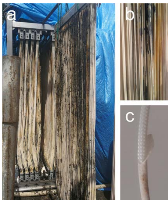
Photo 5. Membranes: a) before cleaning, b) after cleaning, c) visible damage to some fibers (phot. a) M. Kuśnierz , b), c) M. Domańska )
