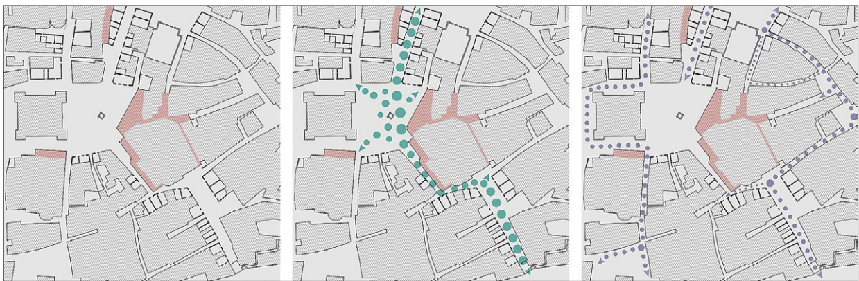
Fig. 4. The area of St. Benedict Square in Norcia, Italy, after the 2016 AVN seismic sequence; from the left: a) urban tissue, b) walkability, c) accessibility for vehicles; by A. Rogulska
