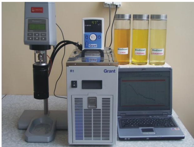
Fig. 2. The researchers post was refurbished with a reometer and tub thermostats
