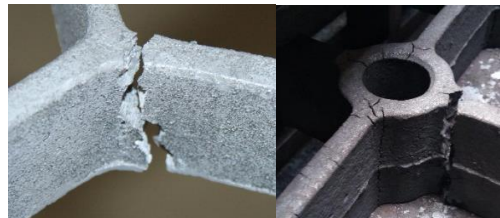
Fig. 2. Cracks formed in grate wall connections
