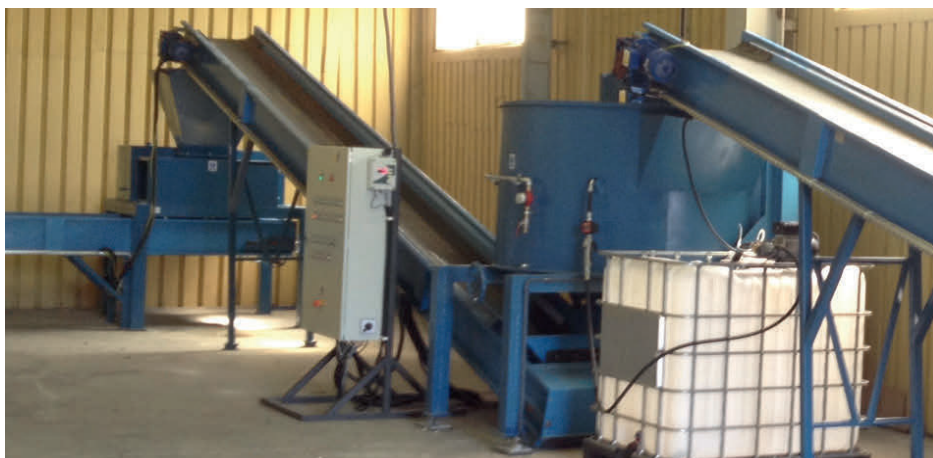
Fig. 1 Industrial line for ferrosilicon briquettes production
