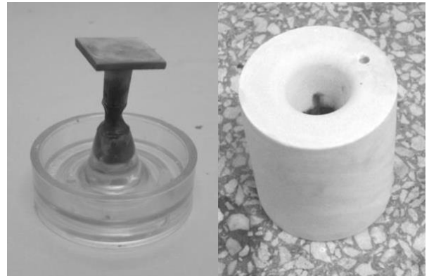
Fig.3. The casting model with nickel coating and ready ceramic mold
