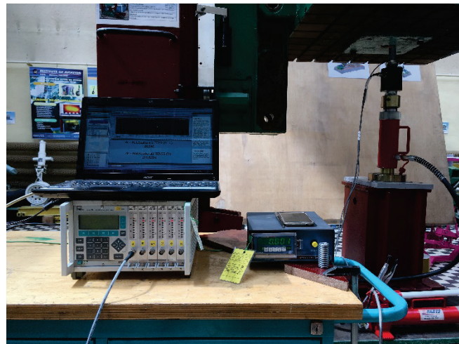
Fig. 5. Pin force measurement system, source ILOT
