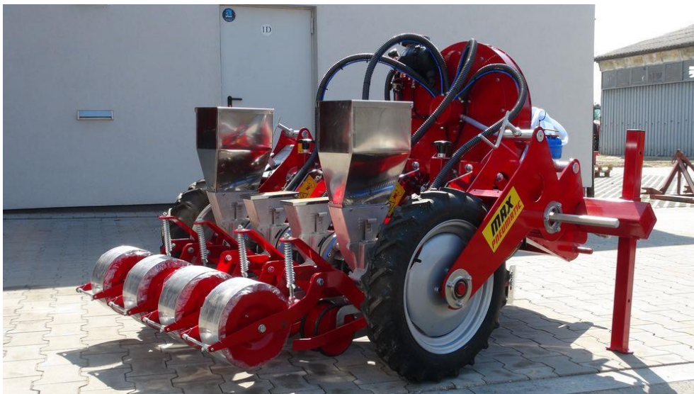
Figure 1. Vegetable seed drill, pneumatic 4-sectional MAX PNEUMATIC ( www.weremczukagro.pl )
