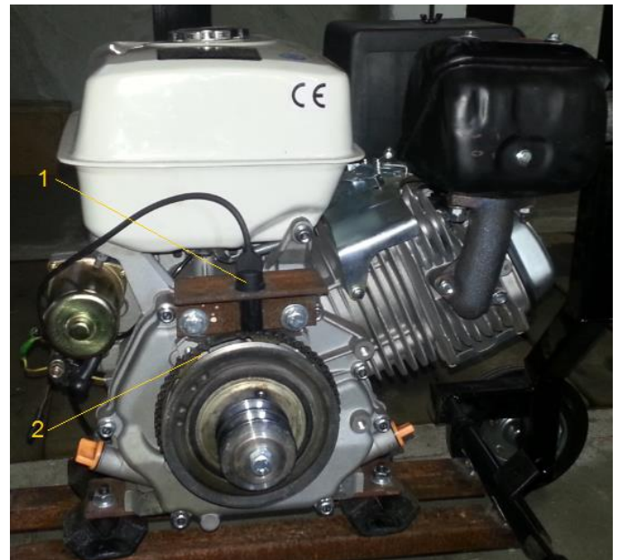
Fig. 8. German spark ignition engine GX390 equipped with: 1- induction sensor, 2 impulse wheel
