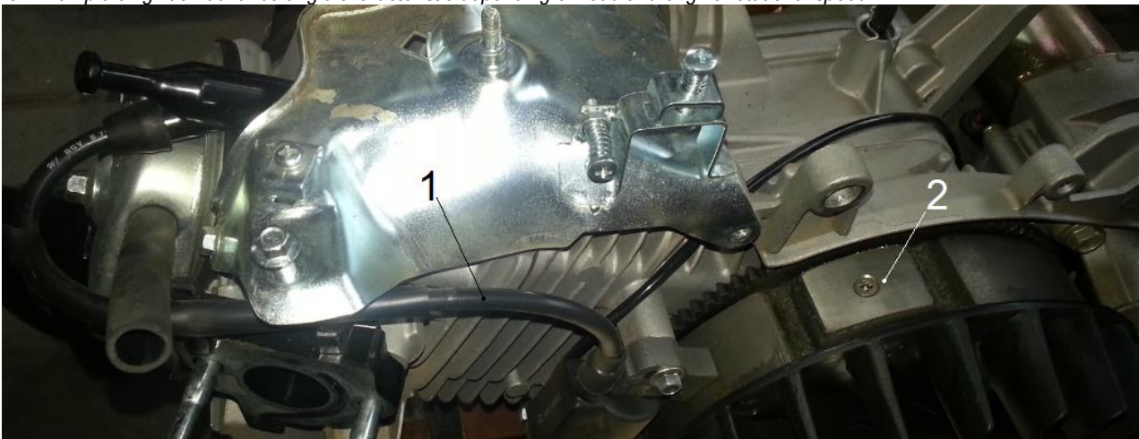
Fig. 5. German engine GX390 engine ignition system where: 1- high-voltage induction and spark-ignition assembly, 2- flywheel magnet inducing high-voltage coil
