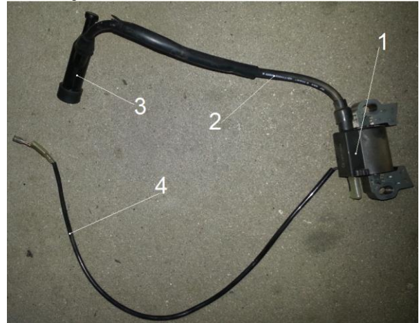
Fig. 4. German GX39 engine ignition system where: 1- Ignition coil with control module, 2-wire high voltage, 3- spark plug, 4-wire ignition signal
