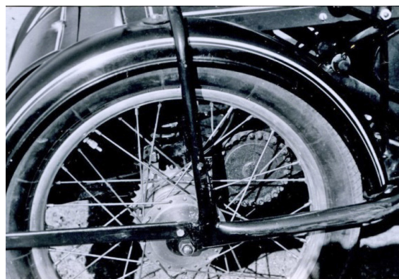
Fig. 8. Manual drive engagement wheel activated by lever on the right hand side [1]
