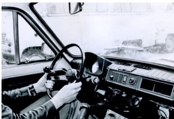
Fig. 22. Clutch disengaged. The lever automatically stays in the lower position [6] Fig. 23. Driver's seat. Pedal cover removed [6]
