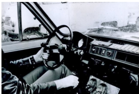
Fig. 20. Manual control. Forward movement of the lever – braking [6] Fig. 21. Manual control – movement of the lever down – disengaging clutch [6]
