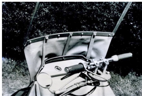
Fig. 12. View from the driver's seat of the steering mechanisms [2]
