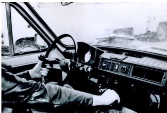
Fig. 20. Manual control. Forward movement of the lever – braking [6] Fig. 21. Manual control – movement of the lever down – disengaging clutch [6]
