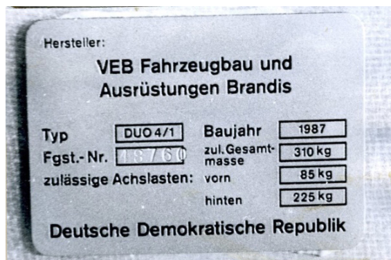
Fig. 32. Data plate, metal, permanently attached to the front wall on the right hand side of the vehicle [4]
