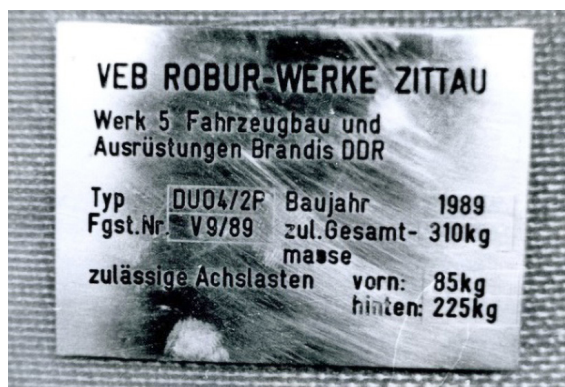
Fig. 37. Data plate, metal, permanently attached to the front wall on the right hand side of the vehicle [5]
