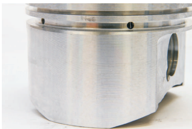
Fig. 2. Piston bearing surface before it was coated with CNT layer
