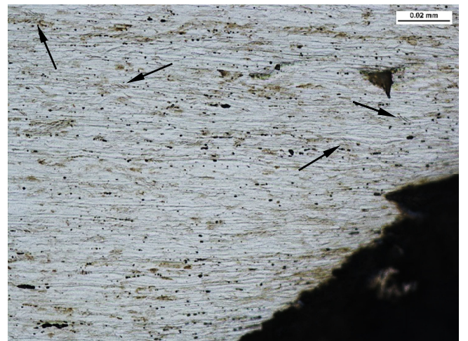
Fig. 13. Microstructure of sample 280°C, LOM, etched in nital
