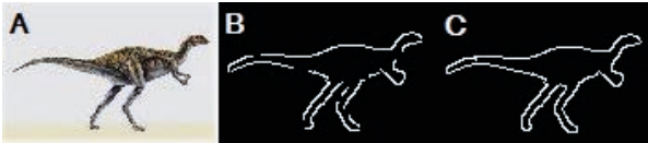
Figure 2. An example of the edge linking process. A - input image, B - edge detection, C - edge linking.
