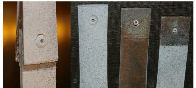
Fig. 3. Final failure of the adhesive-rivet joint
