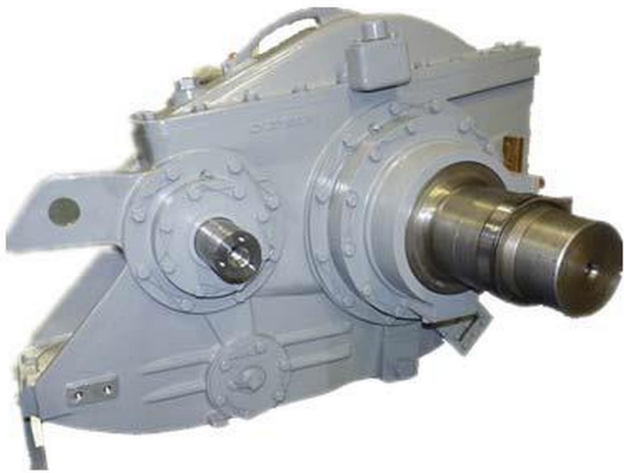
Fig. 1. Gear transmission system of CHR6 intercity train
