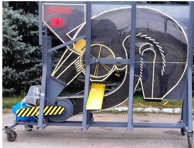
Figure 2. Pneumatic sieve separator for preliminary cleaning of seeds of agricultural crops
