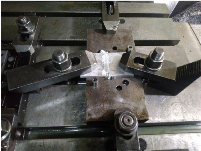
Fig. 2. Experimental setup for FSW of plate
