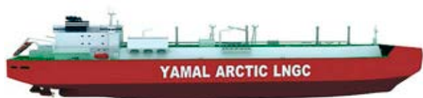
Figure 10. LNG carrier for the Yamal Project, which is powered by 3 azipods and a 45 MW total power (GlobalSecurity, 2021)
