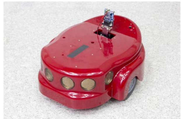
Fig. 1. The Amigobot robot upgraded with a RS232 (the default interface of the robot) – Bluetooth adapter
