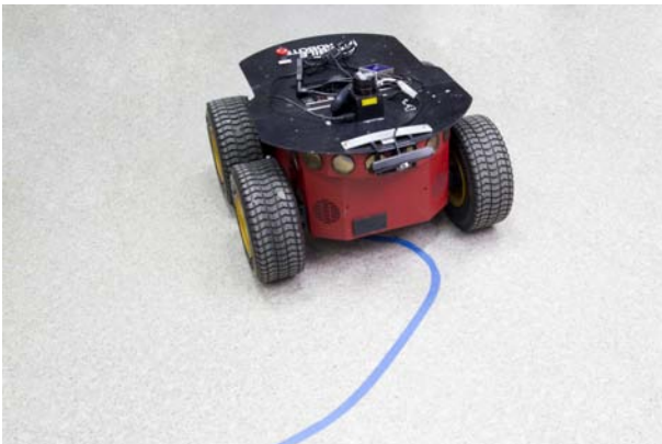
Fig. 4. The 3-DX robot in the camera based line-following exercise
