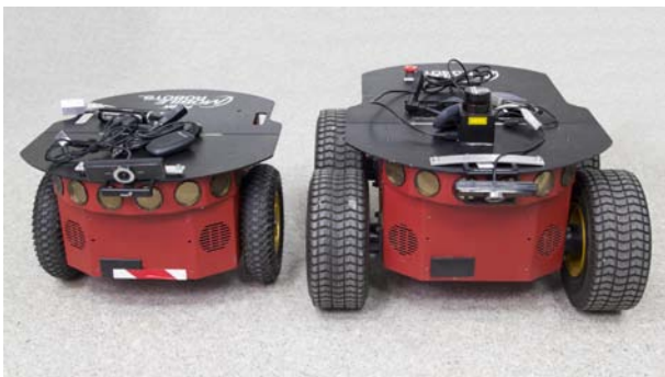
Fig. 3. The Pioneer robots: 3-DX on the left and 3-AT on the right
