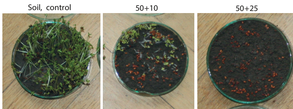
Fig. 5. Lepidium sativum growth on brown soil mixed with oil drilling fluid, sample P-O [25]
