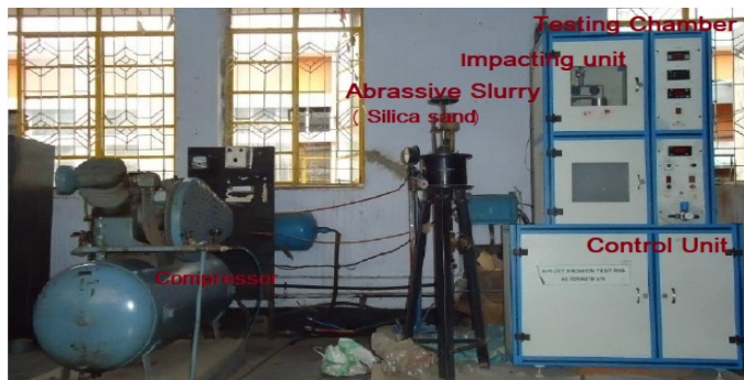
Fig. 2. Set up for Erosion Test
