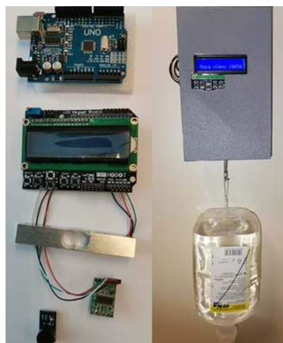
Fig. 1. Electronic components of the scale and the developed concept of the infusion fluid level monitoring system presented in [1].
