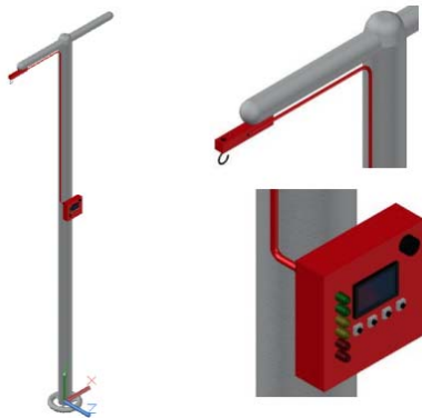
Fig. 7. Model of the splitted monitoring system IV Stand model on the left. Enlarged are: tensometric beam unit in the right upper corner and control unit in the right lower corner.
