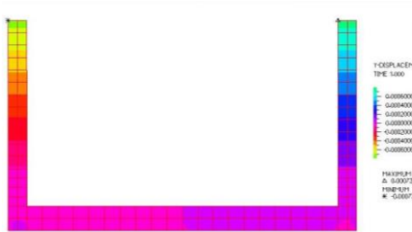
Fig. 4. Horizontal displacement at reservoir
