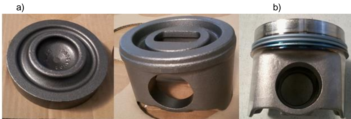
Fig. 1. Subject of the tests a) upper and lower part of the piston b) the piston after welding
