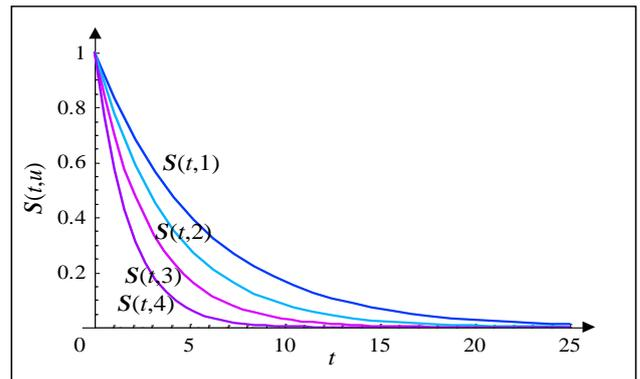
Figure 1. The graphs of a five-state system safety function  $S(t, \cdot)$  coordinates
