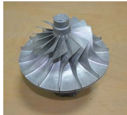
Fig. 4. Turbine compressor rotor casting
