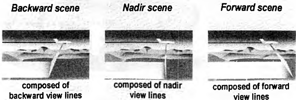
Figure 4. Three-line scanner principle
