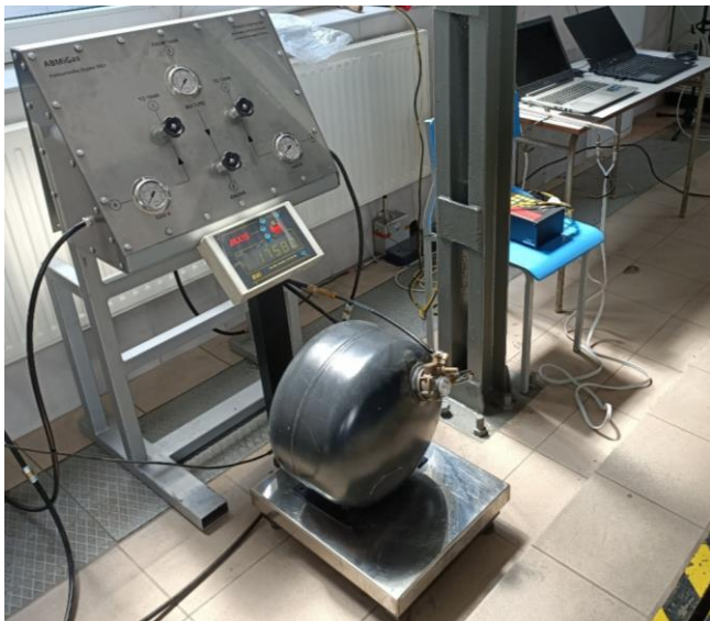
Fig. 2. Stand for preparing of LPG/DME blends
