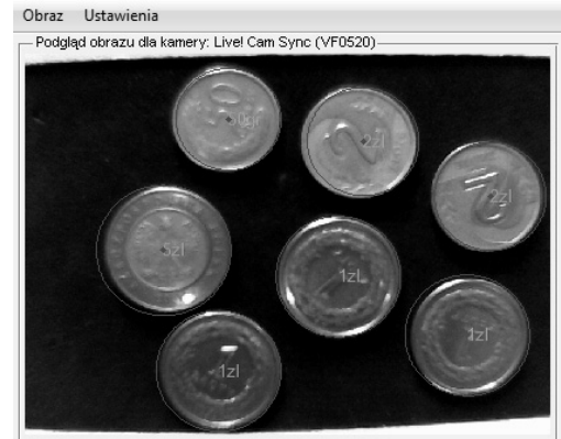
Fig. 7. The result of circular Hough transform operation
