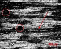
Figure 6. Structure of composite without recyclate made by manual lamination – LR0 (50x) (Panasiuk, 2019)
