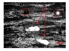
Figure 8. The structure of the composite with a 10% recyclate content, a granulate size of 3.0 mm, made by manual
