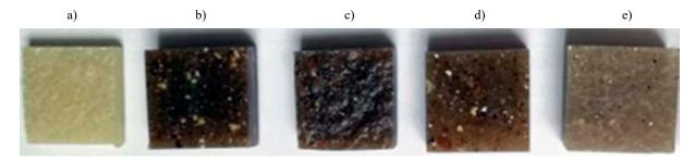
Figure 3. Samples prepared for optical microscopy observation: a) LR0, b) LR20.3.0, c) LR20.1.2, d) LR10.3.0, e) LR10.1.2 (Panasiuk, 2019)
