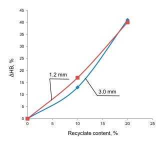
Figure 5. The impact of recycled content and granulation on composite hardness (Panasiuk, 2019)
