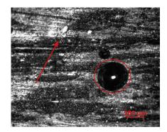
Figure 7. Composite structure with 10% recycled content, granulate size  $\leq 1.2$  mm, made by manual lamination – LR10.1.2 (magnification 50×) (Panasiuk, 2019)
