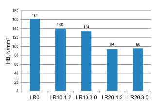
Figure 4. Influence of recyclate content and granulation on hardness (based on (Panasiuk, 2019))
