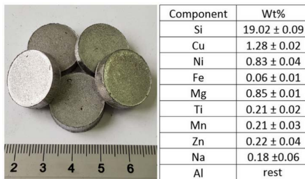
Fig. 2 The appearance of five compacts and its chemical composition
