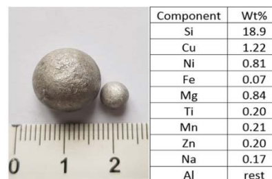
Fig. 11 The appearance of the metal after two-stages cleaning of chips and melting and its chemical composition
