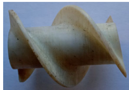
Fig. 4. A sleeve with guiding elements for swirling the injected flow
