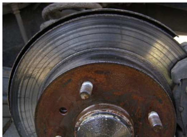
Fig. 4. A heavily worn brake disk in motor vehicle with suspicion of cracks [7]
