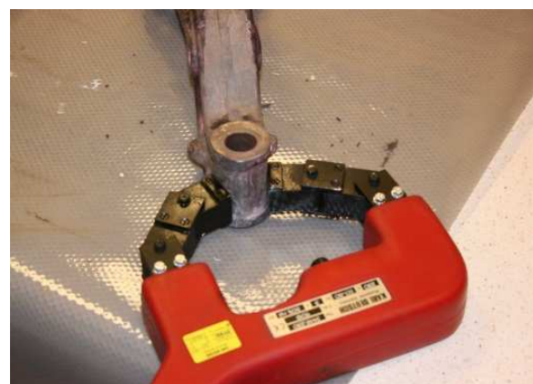
Fig. 11. View of the lever eye of truck suspension tested by the magnetic device using special arms [7]
