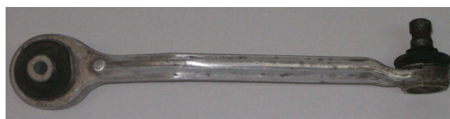
Fig. 5. Deformed arm of independent suspension of automotive vehicle as a result of intensive use or accident [7]
