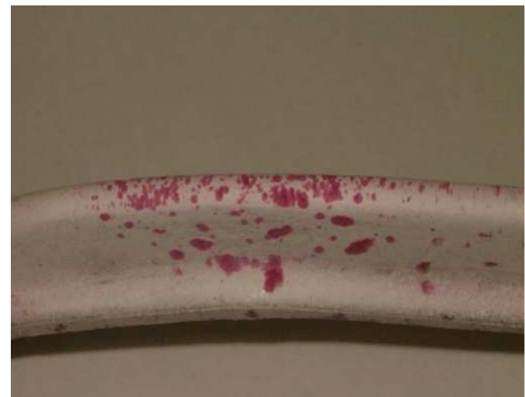
Fig. 10. Another part of the deformed arm suspension with a cluster of discontinuities [7]
