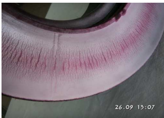
Fig. 8. A fragment of the brake disk tested by coloured penetrant technique [7]
