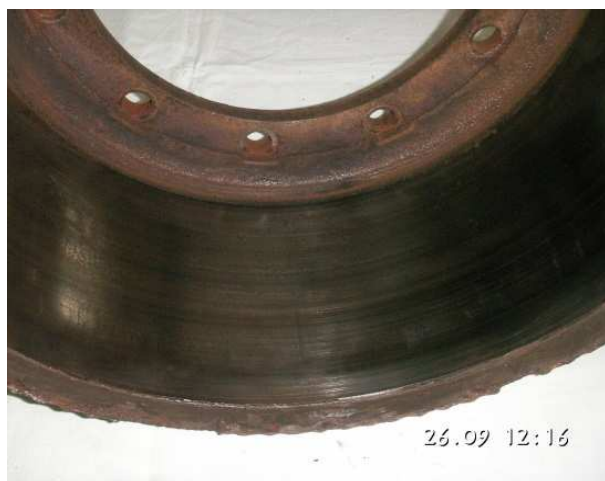
Fig. 3. View of the abrasive worn surface of an exploited automotive brake drum [7]
